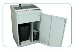
**Convenient storage** After punching, drives slide into the waste bin for storage prior to disposal.
